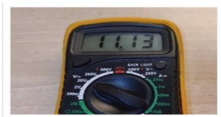
Fig. 5: Battery voltage measurement using multimeter
