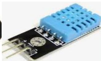
**Fig 3.Temperature sensor**
