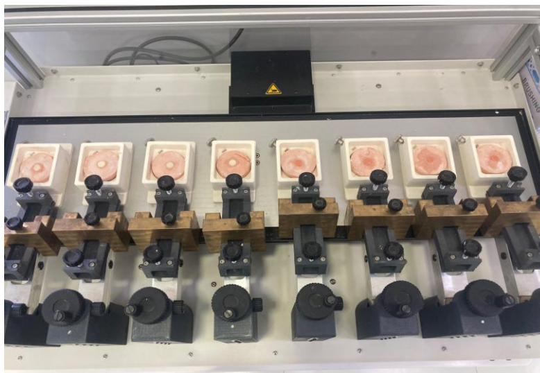
Figure 1: shows the placement of GIC type 2 and 7 in the brushing simulator
