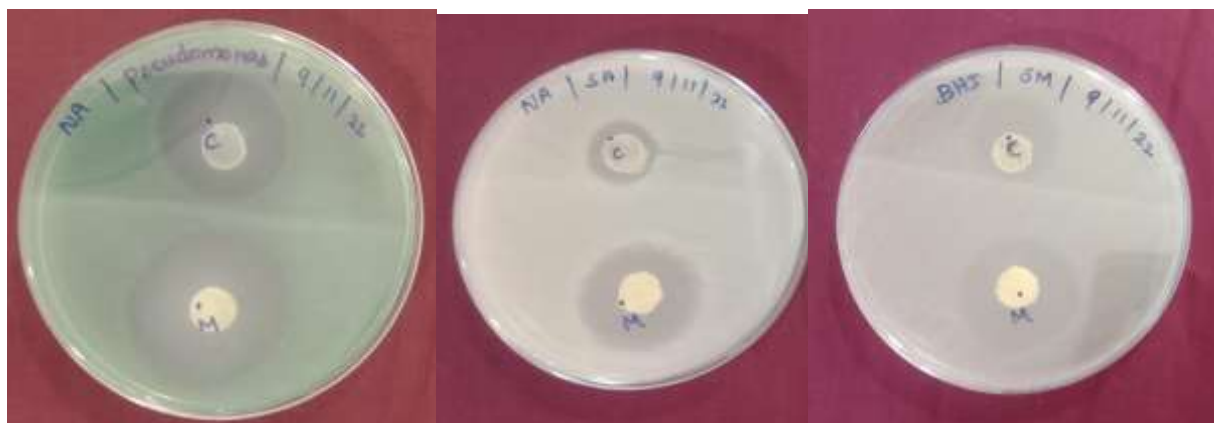
Zone of inhibition of PMMA loaded bone cements with metronidazole against Pseudomonas, S.aureus and S.mutants.
